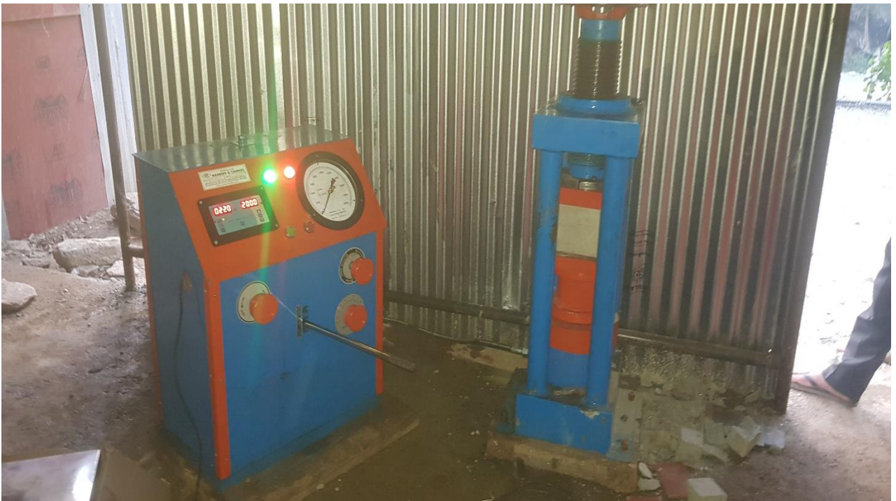
Figure 12: Cube testing at concrete Lab
